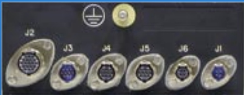
Connectors: Glenair Mighty Mouse 803 Series Bayonet Type
